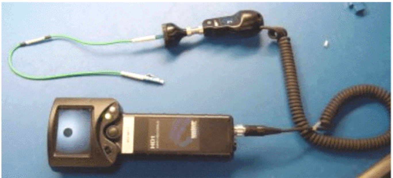
Handheld fiberscope with probe and adapter tip for 1.25mm connector
