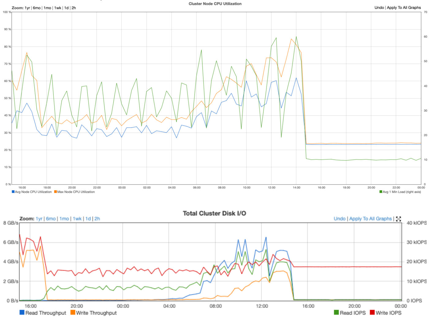
Figure 51 Server Statistic Data Snapshot (CPU Utilization and Disk I/O) from the Controller while Running the GETS 3 Replicas Tests
