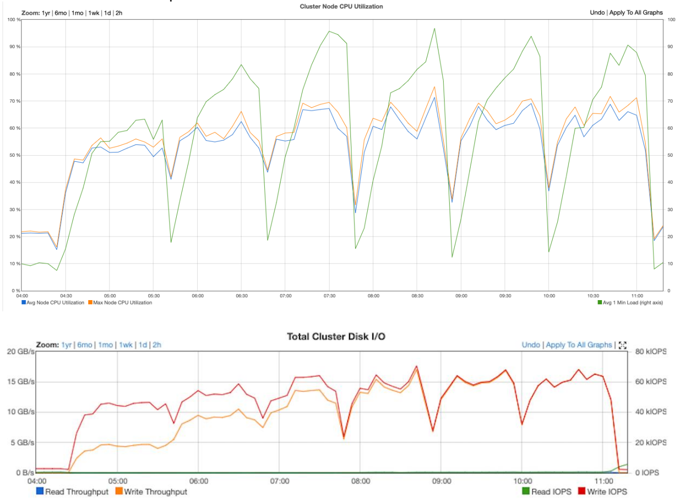
Figure 44 Server Statistic Data Snapshot (CPU Utilization and Disk I/O) from the Controller while Running the PUTS 3 Replicas Tests
