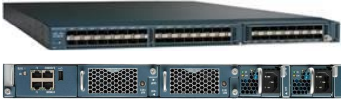
Figure 2 Cisco Fabric Interconnect – Front and Rear
