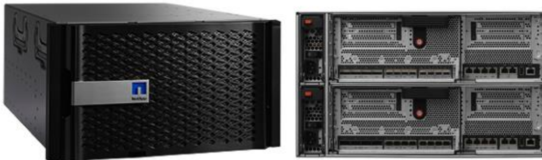
Figure 9 NetApp FAS8040/8060 (6U) – Front and Rear View
