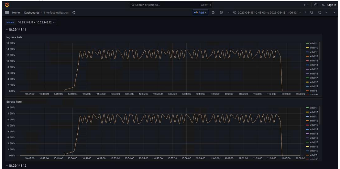
Figure 14. Grafana dashboard monitoring ingress and egress network bandwidth on Cisco Nexus 93600CD-GX leaf 1
