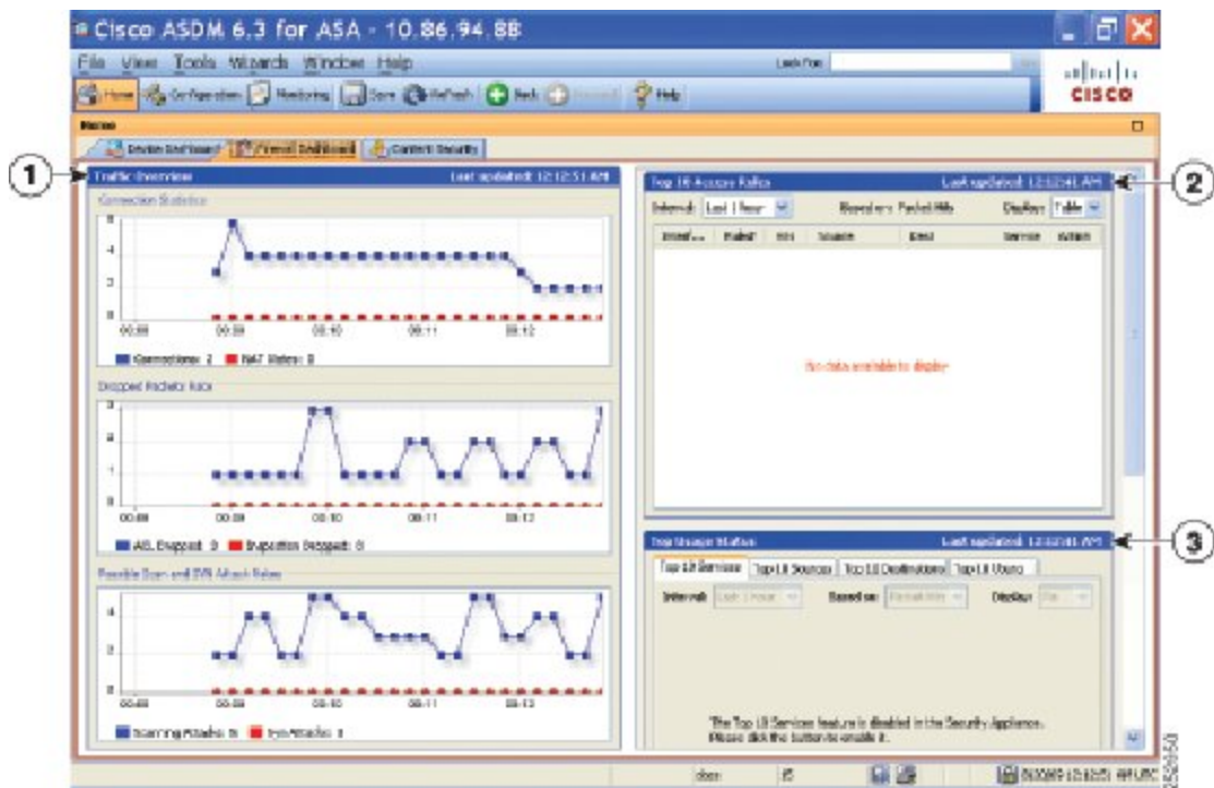
Figure 4: Firewall Dashboard Tab
