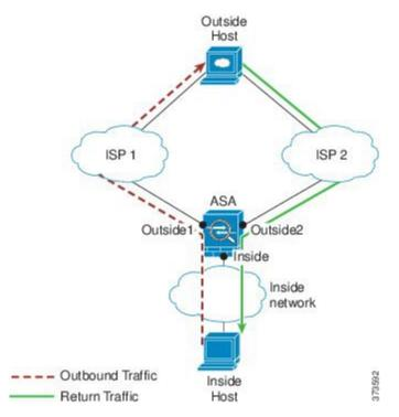
**Non-Zoned Problem**: The ASA maintains the connection tables on a per-interface basis. When the returning traffic arrives at Outside2, it will not match the connection table and will be dropped. For an ASA cluster, asymmetric routing when the cluster has multiple adjacencies to the same router can lead to unacceptible traffic loss.
