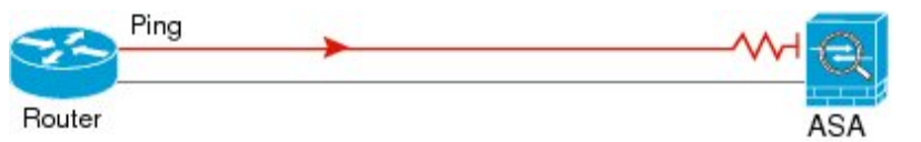
Figure 4: Ping Failure Because the ASA Has No Return Route
