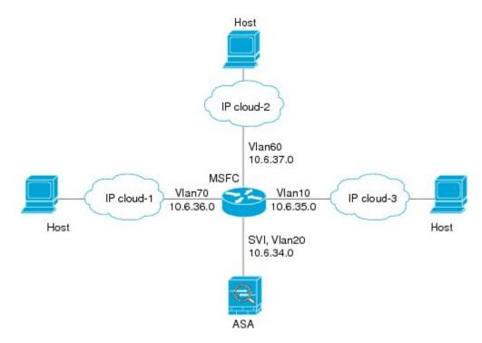
The following sample configuration shows the Cisco IOS **route-map** commands used to enable policy routing in the network shown in the figure:
