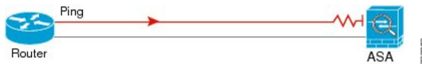
Figure 4: Ping Failure Because the ASA Has No Return Route
