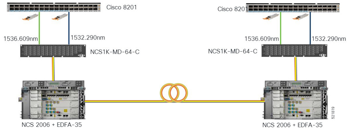
Figure 1: 400G-ZR P2P Short Haul Applications with Cisco NCS 2006
