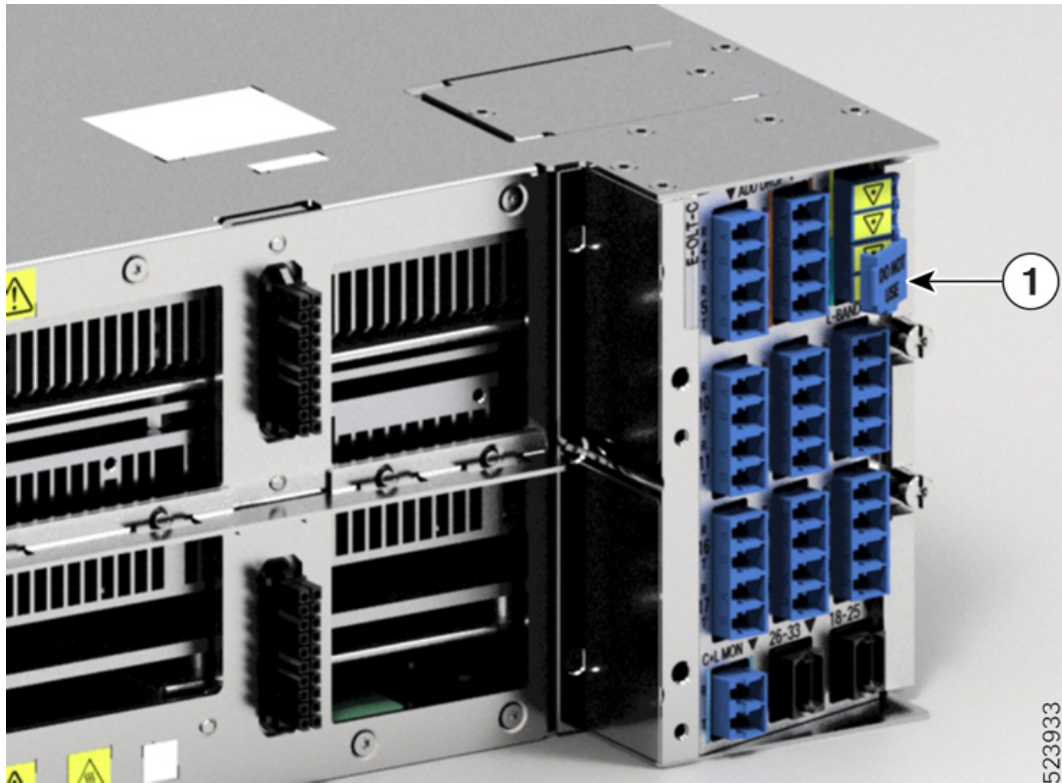
Figure 55: Removing L-Band Cover
