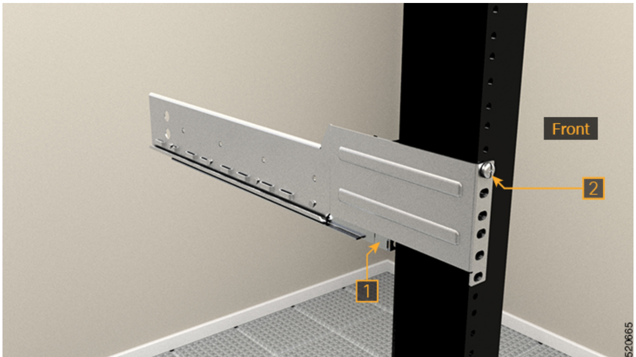
Figure 9: Two Post Slider Integration in the 19" Rack
