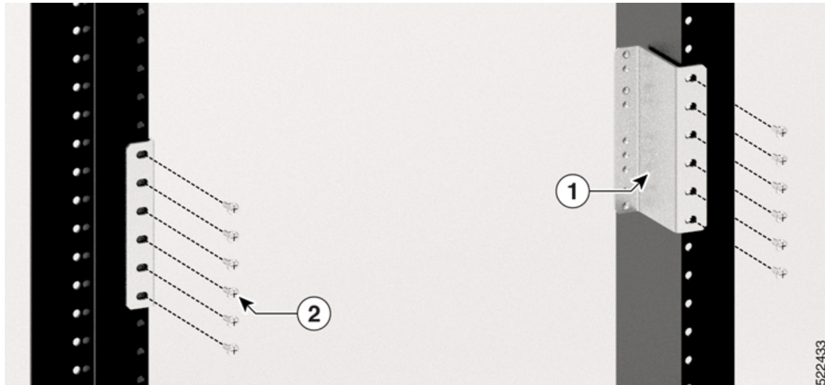
Figure 5: Installing the Adapter Brackets on an ETSI Rack
