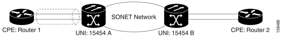
Figure 10-4 LACP Termination Mode Example
