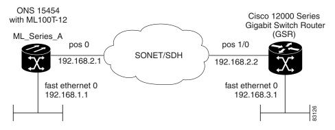
Figure 5-2 ML-Series Card to Cisco 12000 Series Gigabit Switch Router (GSR) POS Configuration
