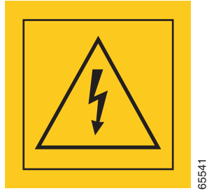
Figure 4-31 Electrical Energy Hazard Label
