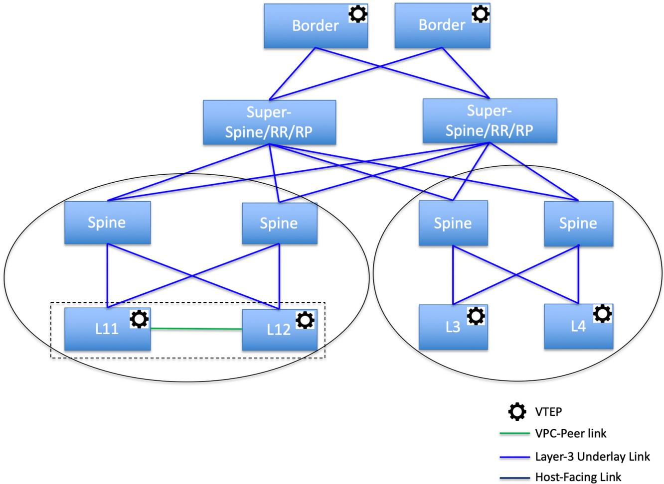
In this topology, there are four leaf switches connecting to the spine switches, which are connected to two super spine switches. These super spine switches are connected to the border or border gateway leaf switches.
