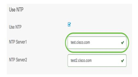
Step 16. (Optional) Enter a second NTP server address in the *NTP Server2* field. This serves as a backup in case NTP Server1 fails to sync to the network. A green checkmark will appear in the field if the entered NTP server address is valid.
