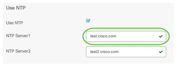
Step 17. (Optional) Enter a second NTP server address in the *NTP Server2* field. This serves as a backup in case NTP Server1 fails to sync to the network. A green checkmark will appear in the field if the entered NTP server address is valid.
