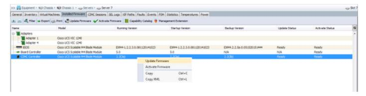
3) Select the correct firmware, the Force checkbox and click Apply.
