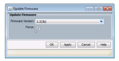
**Tip**: If it's not clear which version needs to be selected from the dropdown, the server administrator can navigate to **Equipment** > **Firmware Management** > **Packages**, expand ucs-k9-bundle-b-series. *VERSION*.B.bin and look for "ucs-EXM4." There will be three components: bios (BIOS), brdprog (Board Controller), and cimc (CIMC Controller).
