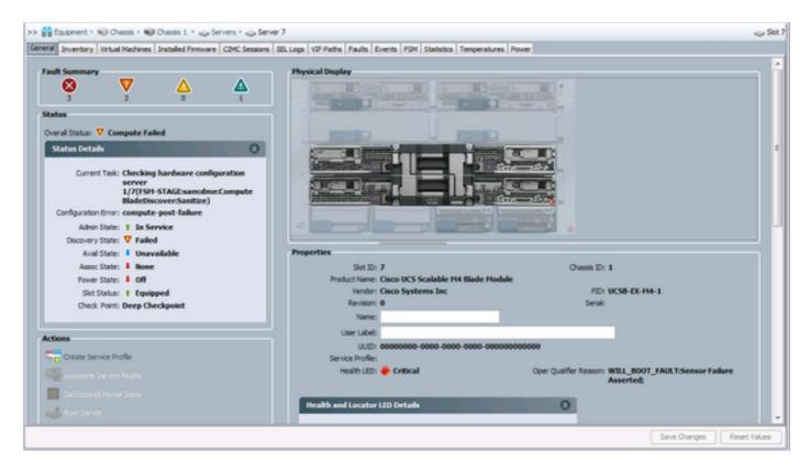
The POST Results can be verified by clicking the **View Post Results** under *Actions* in the **General** tab. The figure below shows that the problem is due to a CPU Mismatch.
