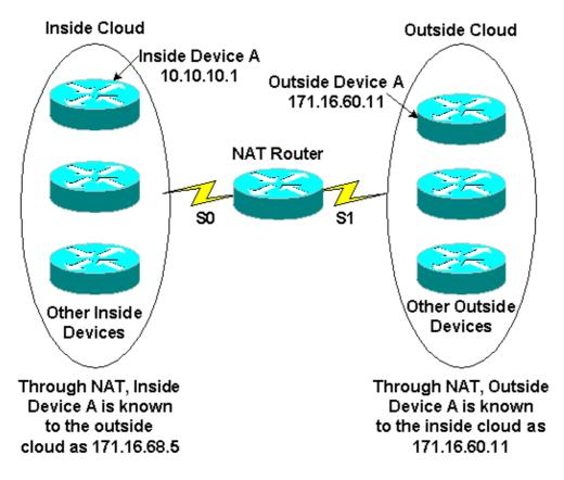
NAT is generally used to conserve IP addresses routable on the Internet, which are expensive and limited in number. NAT also provides security by hiding the inside network from the Internet.
