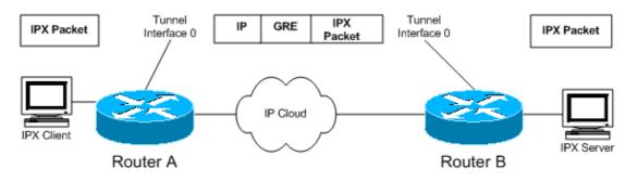
As illustrated in the diagram, GRE tunneling can also be used to encapsulate non–IP traffic into IP and send it over the Internet or IP network. The Internet Packet Exchange (IPX) and AppleTalk protocols are examples of non–IP traffic. For information on configuring GRE, see "Configuring a GRE Tunnel Interface" in Configuring GRE.
