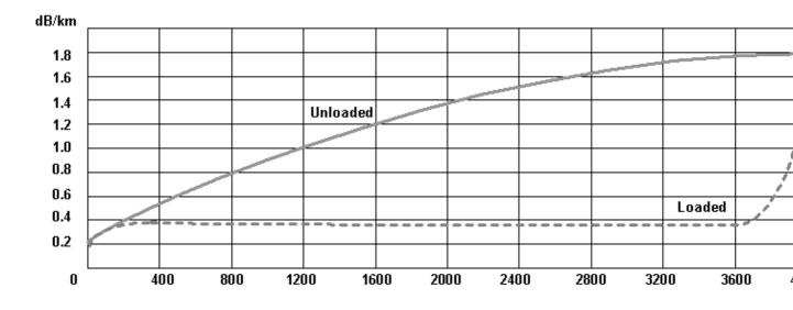
With a load coil, the three-mile loop discussed above reveals a roll-off point at around 3300 Hz only.
