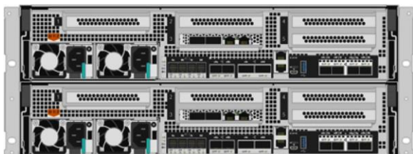
Figure 14. NetApp AFF A400 rear view
