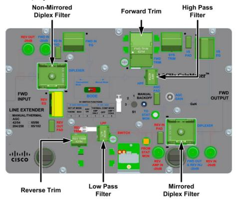
Install two (2) new diplexer, being careful to match the location of "mirrored" and "non-mirrored" diplexer.
