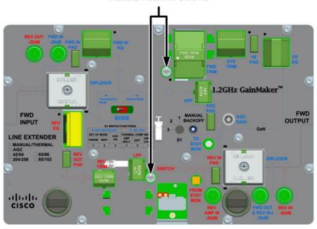
4 Remove the line extender module from the housing.
