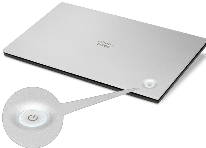
Power button with LEDs encircling the button
