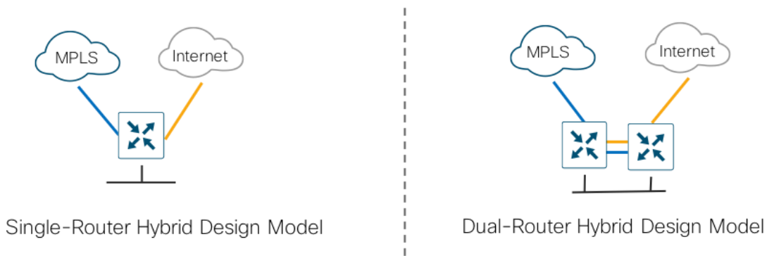
Figure 14 Single-router and dual-router hybrid design models
