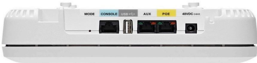
2. Use a standard Ethernet cable and connect the LAN port off your broadband modem or router directly to Ethernet port marked "POE" on the access point.
