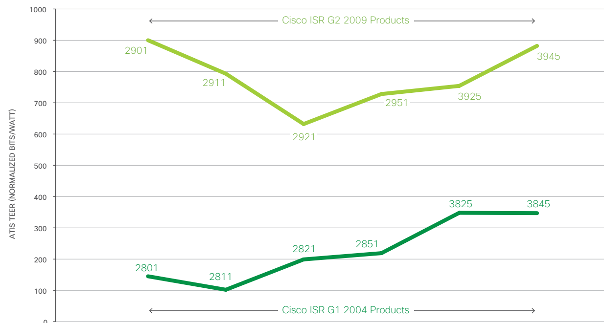
Figure 4: Energy Efficiency Performance Improvements Between Two Generations of Cisco Integrated Services Routers
