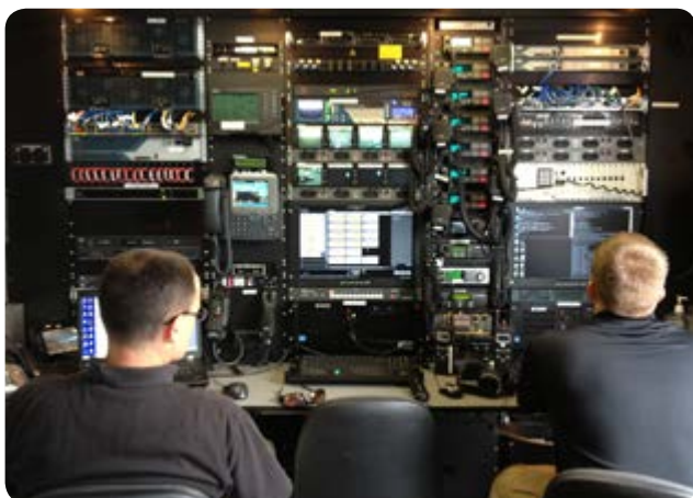
The Cisco Network Emergency Response Vehicle (NERV) is a mobile communication center, supported by a highly trained team, that is designed to establish interoperable communications in emergency situations.
